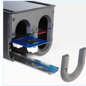
removable end caps and floor allow for the removal and changing of power/data plates
